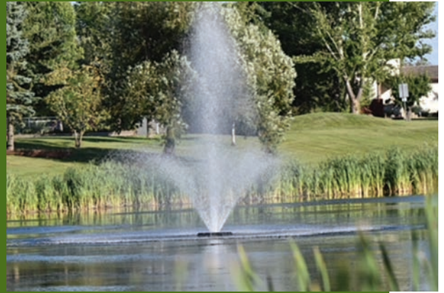
Aerating fountain installed at Sunshine Lakes Pond.
