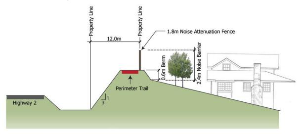
Note: The berm and sidewalk along the highway buffer varies longitudinally, as the trail will not always be on top of the berm in certain areas where Highway 2 and the CN Rail intersect.
