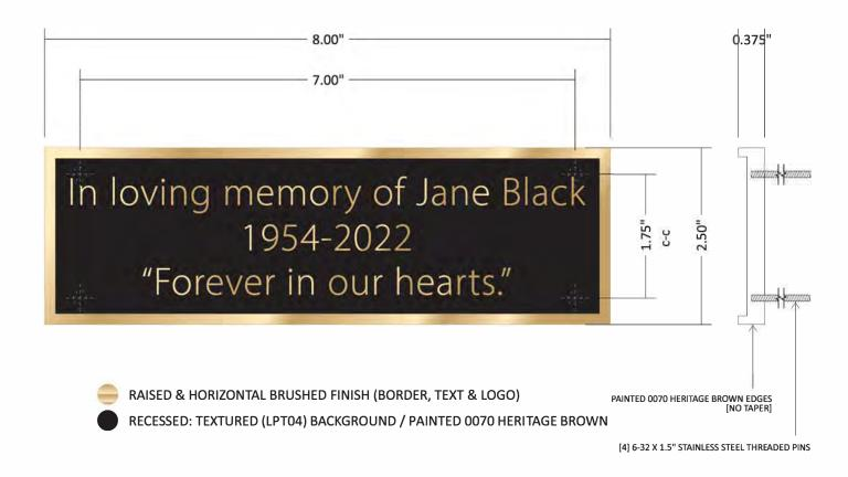
Signage Elevation & Section SCALE 1:1.5
